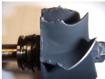
Damaged exhaust turbine
