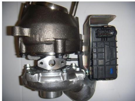
Once mounted on the vehicle, the turbo may not function correctly. This is because the ECU or DDE needs to be reprogrammed by the authorised technical service in order to function correctly, given the fact that the position regulator and the diagnostics are both incorporated in the servomotor.
