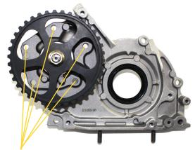
The bolt holes are accessible: Pulley removal is not necessary
