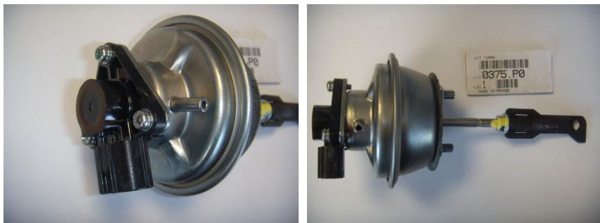
This sensor is prone to a function error (error: electronic sensor re-copy turbo-charger geometry position)
