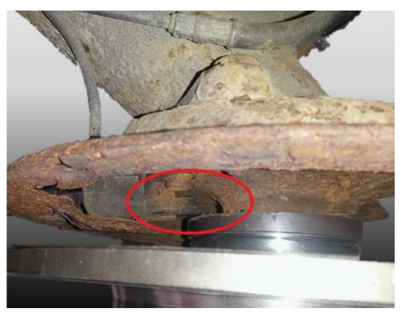
The solution is to remove the ABS sensor from its mounting point and remove any corrosion before refitting the ABS Sensor and new disc.
