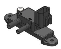
You will notice the design of the SMPE manufactured exhaust pressure sensor differs from the original unit. The OE design uses a ceramic capacitive device which is prone to early life failure and is less accurate than the modern electronic pressure sensor used in our redesigned unit. We were able to repackage the electronic sensor and attach it to a mounting bracket, ensuring the same footprint as the original design
