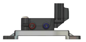
Although the orientation of the outlet pipes has been rotated through 90 degrees, the diameters of the pipes have been retained, so you will encounter no problems fitting the original mating pipes to our unit. The colour coding in the above diagram helps you to fit the mating pipes correctly
