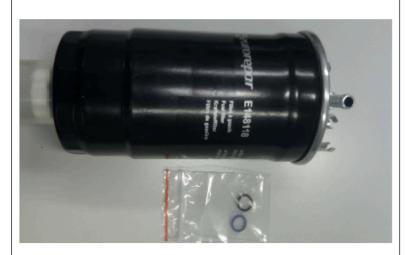
1. Locate the two O rings supplied with the filter for the thermostatic valve.
