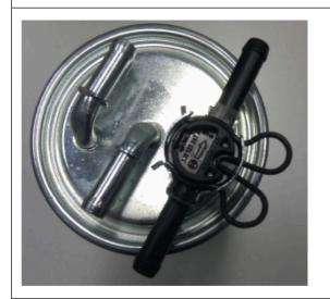
3. Lubricate the O rings with diesel fuel and locate into the housing securing with the retaining clip.
