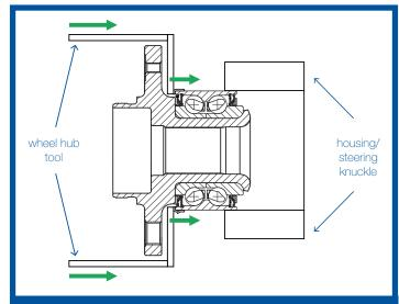
The correct special tool should be used to avoid damage to the inner structure of the bearing. The force should be applied to the outer race of the bearing.
