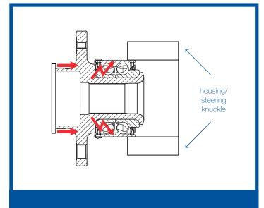
This shows incorrect installation process which leads to the problems mentioned above.
