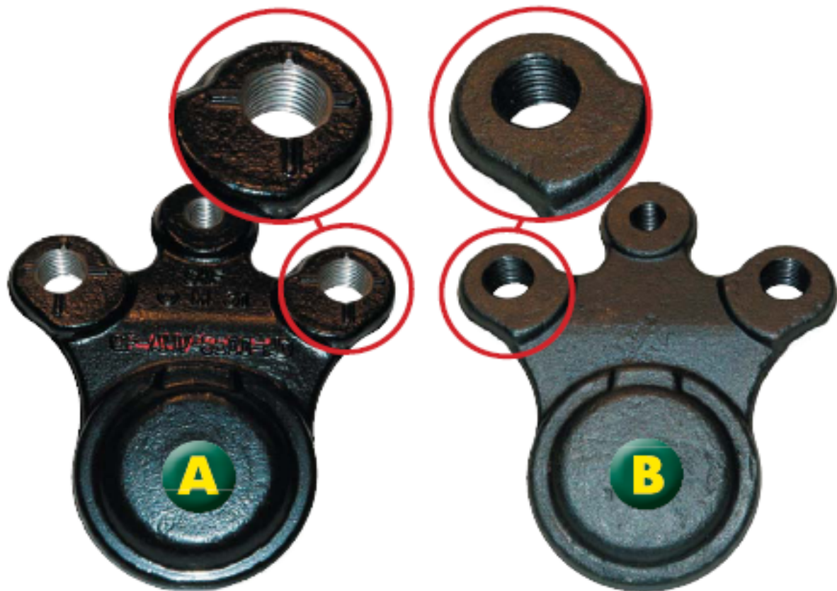
FIRST LINE / OE PART incorporating locating mechanism and OE bearing & seal
