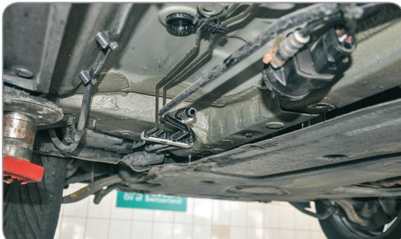
**EN** Remove fuel filter, replace clamping ring from used filter to the new filter and fix new filter
