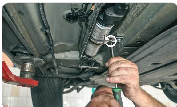
EN Loosen filter clamping ring
