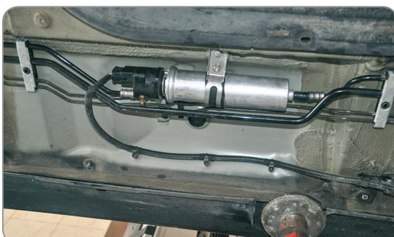
**EN** Start the engine, check system for leakage, fix chassis masking elements
