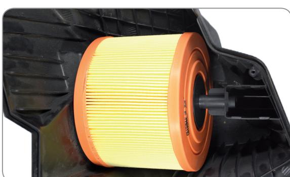
EN Properly installed a filter. Close and fasten the housing cover
