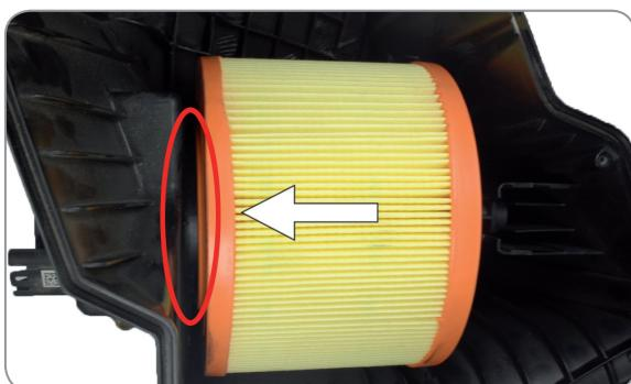
EN Push the filter on flange in the housing
