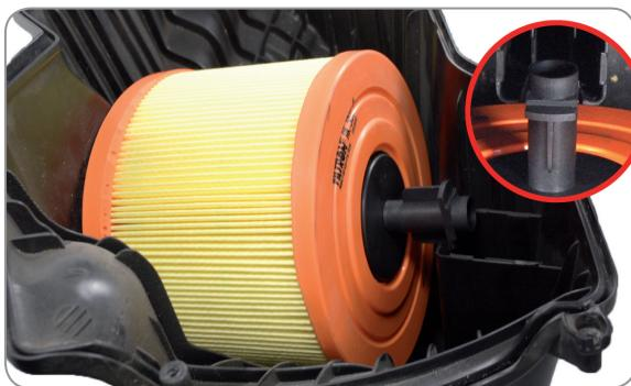
EN Open the housing and remove old filter, then place the new filter in the housing
