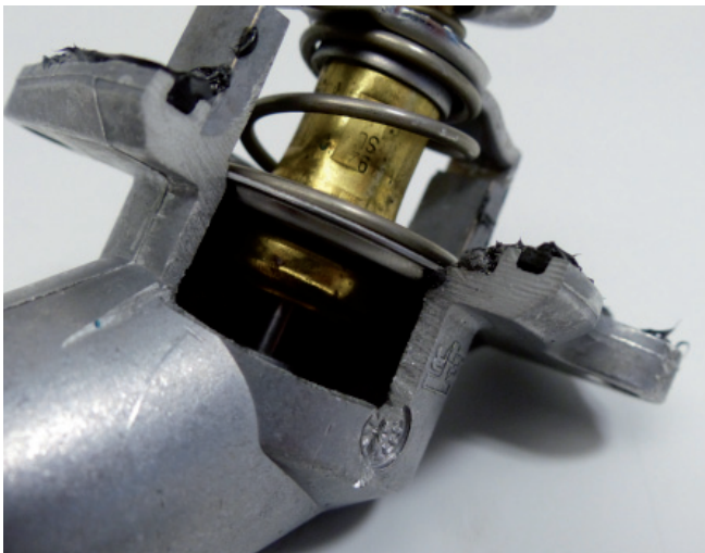
The application of sealant has led to the thermostat no longer sealing properly.
