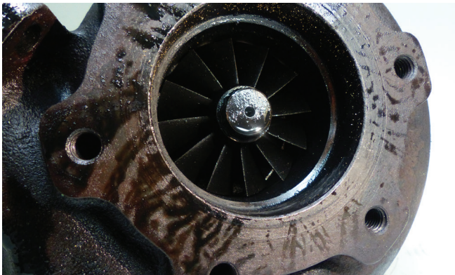
Figure 1: Oil at the turbine outlet of the turbocharger
