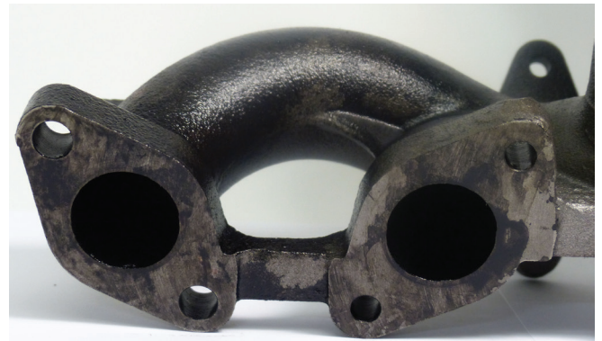
Figure 2: Oil enters at the turbine inlet
