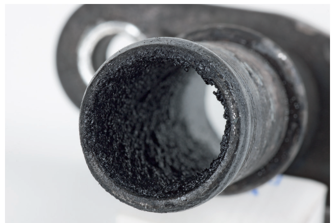
Figure 4: Coked oil return line as a result of exhaust gas penetratio
