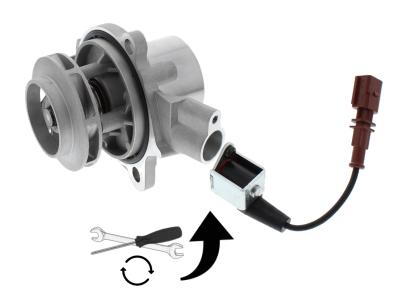
Please note: It is important to re-connect the solenoid to avoid an error message or warning light displaying on the instrument panel.
