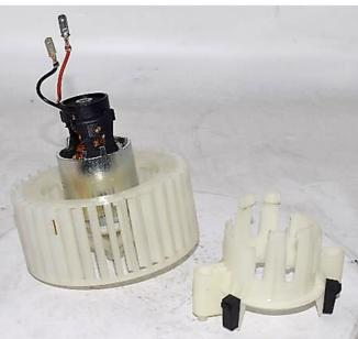
8) Use new interior blower (ERA 664089) and put together each parts, following the reverse process.
