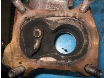
Gasket correctly mounted.
