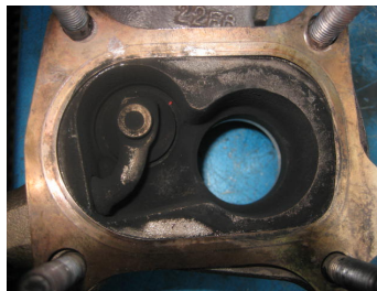
Gasket incorrectly mounted
