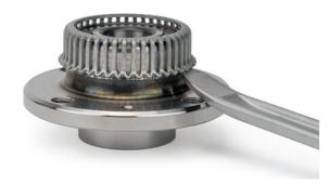
Image 2: The sensor ring must be removed if the wheel bearing is installed in vehicles without ABS. This can be done using a tyre lever, for example.
