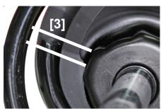
Correct spring position: the rubber bend and the end of the spring are in line [3].
