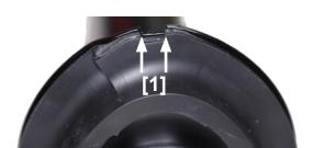
Align the groves of the McPherson strut and the rubber plate [1]
