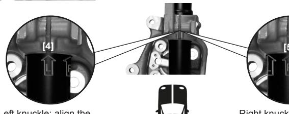
Left knuckle: align the shock absorber with the arrow "L" into the centre of the groove [4].
