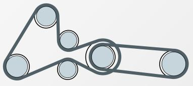
**Fig 2** - Auxiliary drive diagram (from engine No. 0113090), fitted with the elastic multi V-ribbed belt 70 94 0717.
