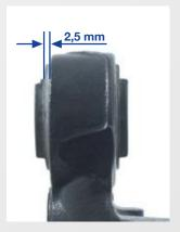
The slot in the new rubber mount must be aligned with the marking on the trailing arm, then installed with a suitable special tool until the mounting is pressed in, up to the dimension of 2.5 mm.
