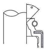
↑ Sealing lip radius (R) → ↑ Lubrication ↑ Sealing Lip contact angle (a) → ↓ Lubrication
