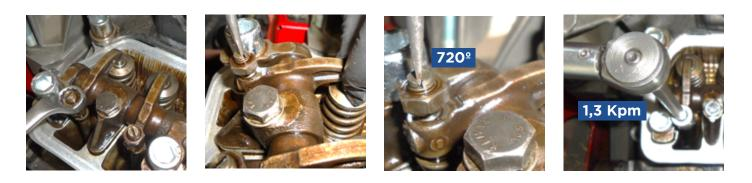
**3.** Tighten the bolt again until completely eliminate the clearance between the rocker and the valve.
