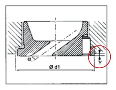
Maximum distance for the machining of the prechamber housing.
