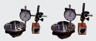
Check the contact surfaces of the wheel hub for deformations with a micrometer clock (Max. fling 0,03 mm.)
