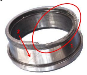
These small pieces of broken metal then find their way into the bearing raceways, this soon results in a noisy bearing and eventually the premature failure of the bearing.
