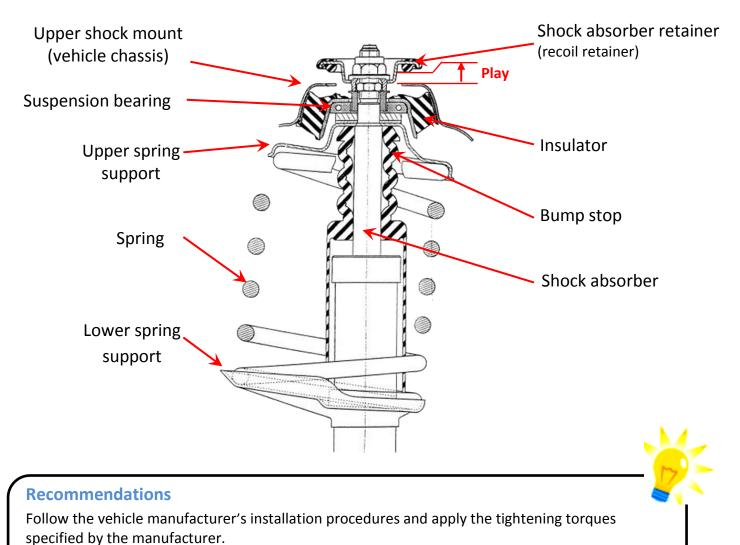
We recommend replacing suspension bearing kits in pairs.
