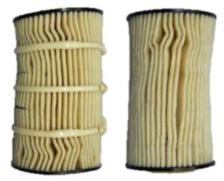
Both filters have been pressure and performance tested. Picture shows collapse pressure test whereby both filters show same structural and visual damage. Glue beads break after 2bar of pressure.
