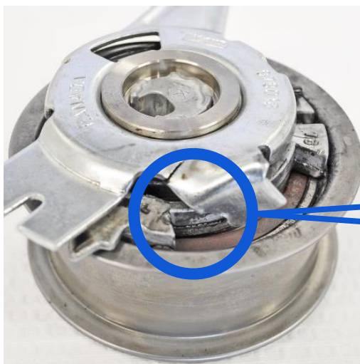
The back plate is severely deformed and torn.
