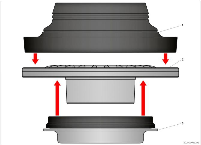
Fig. 1: Assembly of the suspension-strut mount (example)
