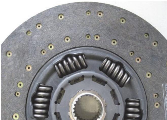
Fig. 3: Lining on the gearbox side
