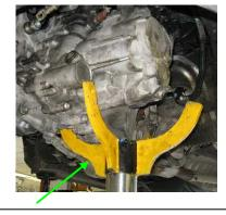
Use the appropriate device to assembly and disassembly the gearbox. The operator never must support the weight of gearbox.
