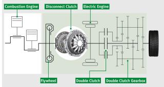
Image 1: System design of the plug-in hybrid drive
