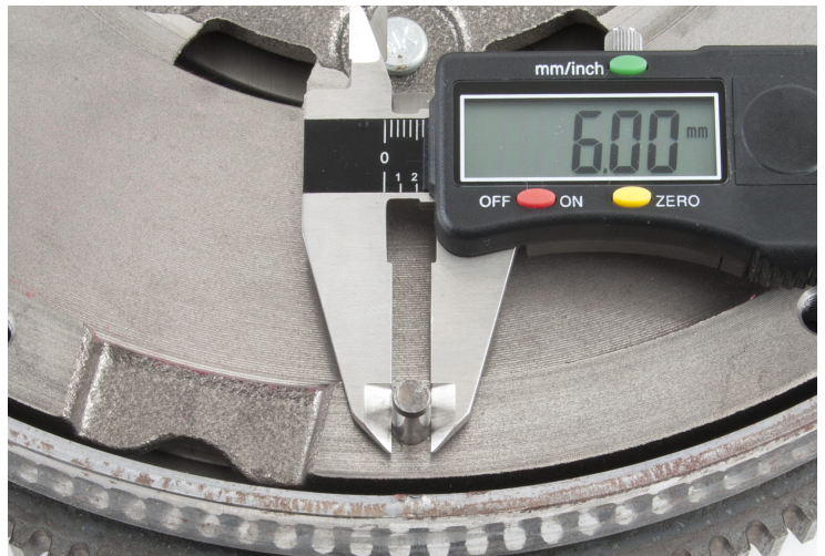
Fig. 1: Measuring the diameter of the centering pin
